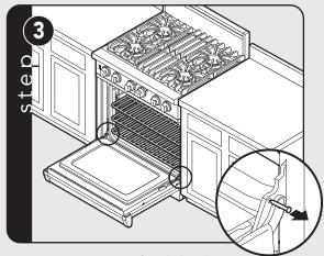
Remove pins from hole in hinges.
